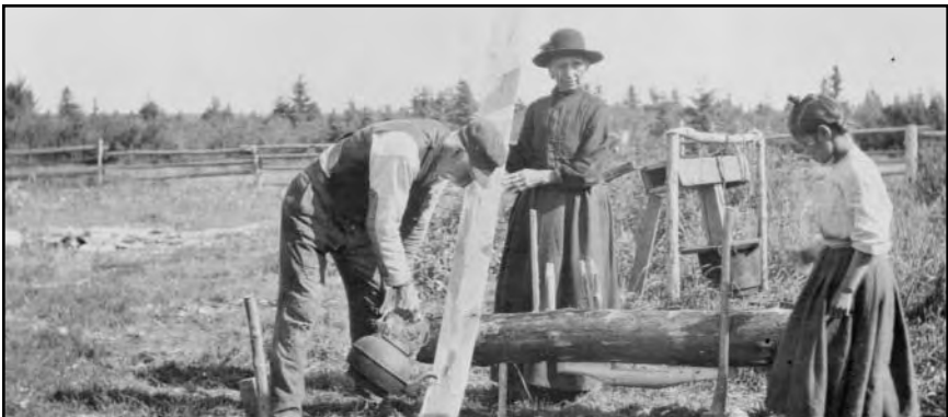
Malecite Indians bending the plank to make a toboggan, [Burnt Church, NB], before 1936. Photography by Canada, Dept. of Mines & Technical Surveys. Library and Archives Canada, negative PA-041760
